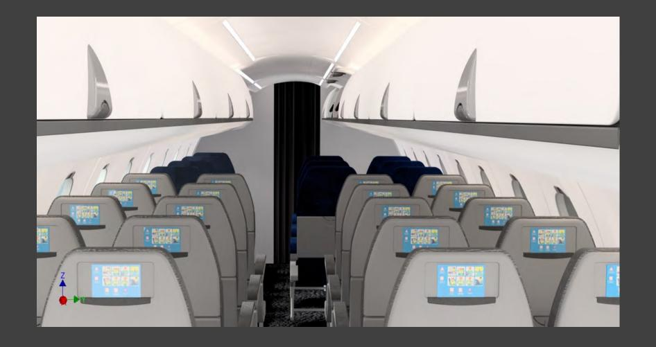
The current CRJ 700/900 Classic overhead bins cannot accommodate a standard carry-on bag. Instead, this baggage is gate checked and placed in the baggage bay. Passengers must wait in the jetway after the flight to retrieve their bag. The crew can't head to their next assignment until all passengers are clear.
